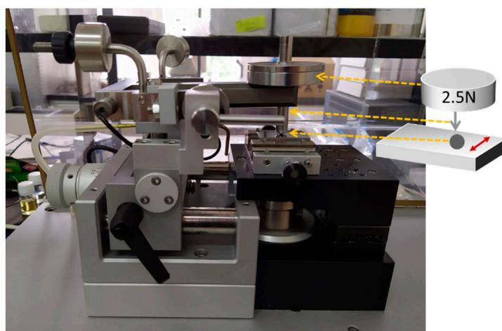
Figure 6. Tribological experimental setup for reciprocating tests.
