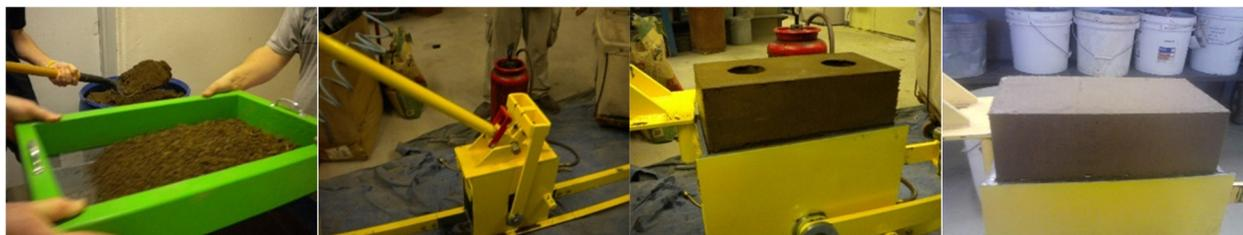
**Figure 8.** Process of CSEB making.
