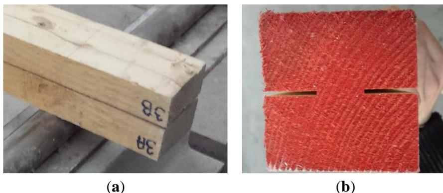
**Figure 7.** (a) Timber beams cut in half; (b) Notched beams.
