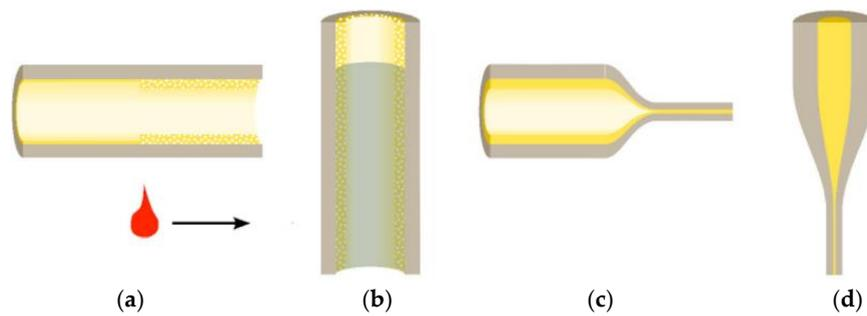
**Figure 3.** Principle of the preparation of the rare-earth-doped fiber by MCVD and solution doping method: (a) deposition, (b) solution doping, (c) collapsing, and (d) fiber drawing. Adapted with permission from [142], W. Blanc and B. Dussardier “Formation and applications of nanoparticles in silica optical fibers”, *J. Opt.* **2016**, *45*, 247–254. Copyright 2015 The Optical Society of India.
