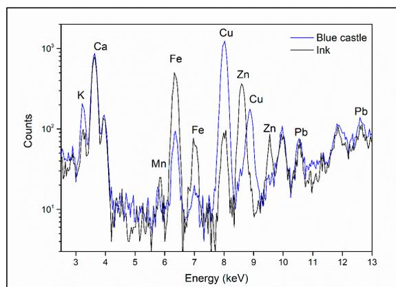
**Figure 7.** Graph with selected XRF spectra. **(blue line)** The blue castle in West Africa is drawn with azurite (Cu) and green earth (K, Mn, Fe); **(black line)** High Fe peaks confirm the use of iron-gall ink.
