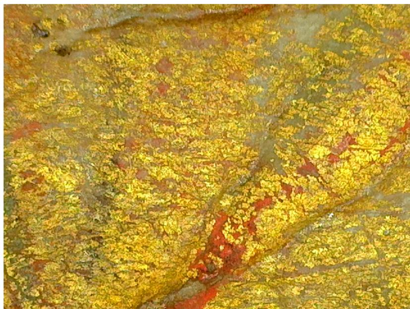
**Figure 9.** Gilded wind rose observed under digital Dino microscope. Gold foil was placed on a transparent *mixture* (reproduced with permission from the AGI).
