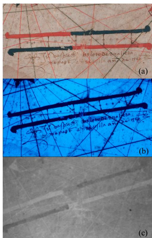
**Figure 5.** (a) Visible image of the scale bar with the signature and the date. (b) UV image of the same area and (c) IRR image of the same area; the inscription is not visible under IR, indicating the use of iron-gall ink. White lines and bands correspond to vermillion; dark bands to azurite, probably underpainted with carbon black; thin black lines to a copper-based green pigment, as confirmed by XRF.
