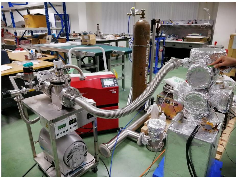
Figure 9. Checking for leaks in the vacuum system.
