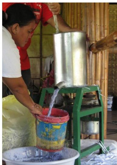
**Figure 2.** The pulping machine utilized during briquette production showing the wet pulped paper produced.
