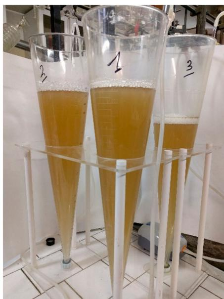
**Figure 2.** Experimental setup of the struvite precipitation process.
