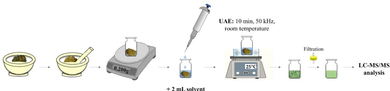
**Figure 2.** Schematic representation of the UAE experimental procedure.
