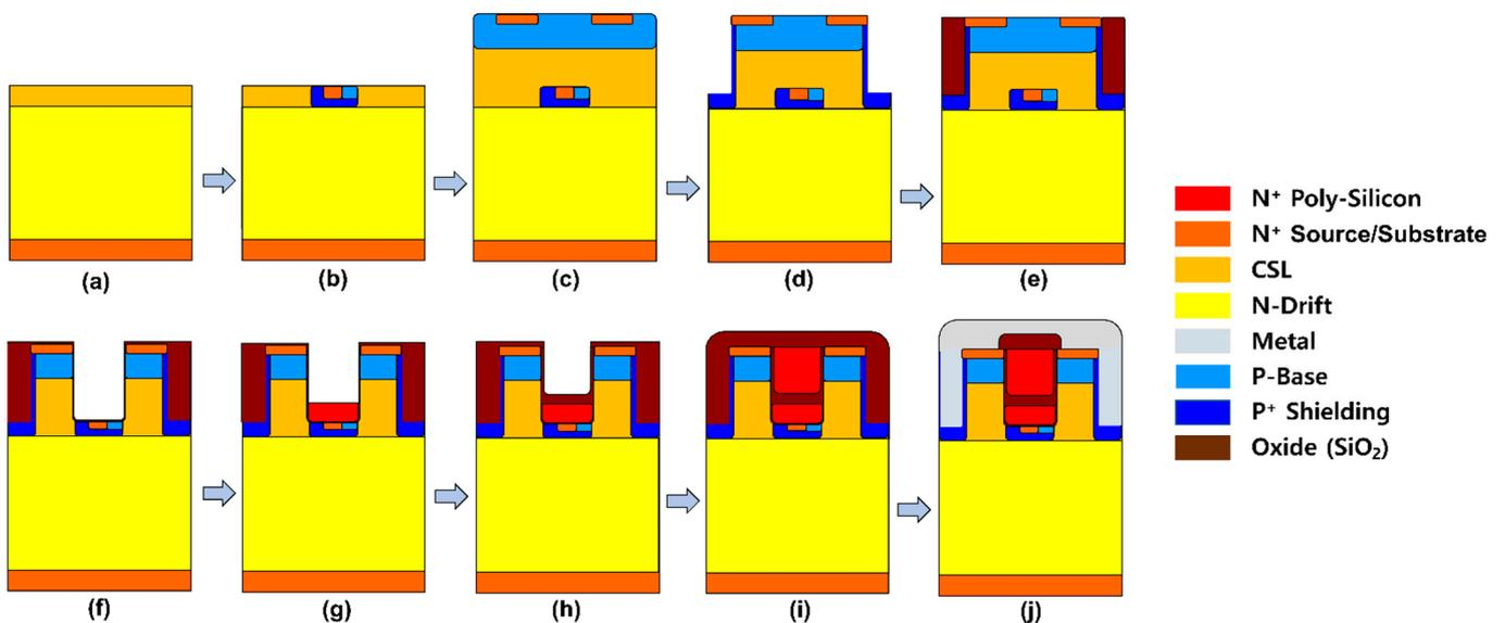
**Figure 3.** Proposed fabrication procedure of DTMCD-MOSFET. (a) N-drift region and CSL region formed by epitaxial growth on N+ substrate. (b) BPR region formed by ion implantation. (c) Left CSL
