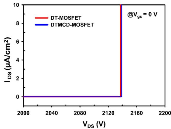
Figure 7. Comparison of off-state characteristics of DT-MOSFET and DTMCD-MOSFET.
