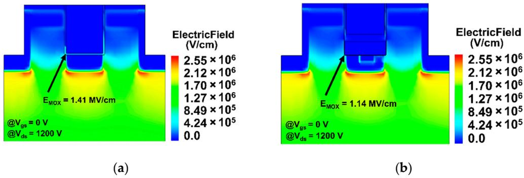
Figure 8. Cross-sectional view of the electric field distribution of (a) DT-MOSFET and (b) DTMCD-MOSFET at  $V_{DS} = 1200$  V.
