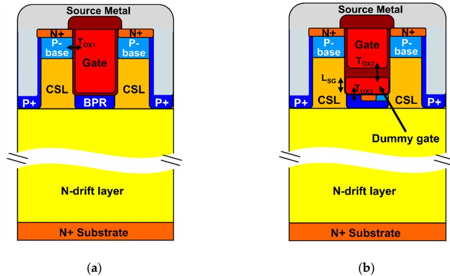
Figure 1. Cross-sectional view of (a) DT-MOSFET and (b) DTMCD-MOSFET.
