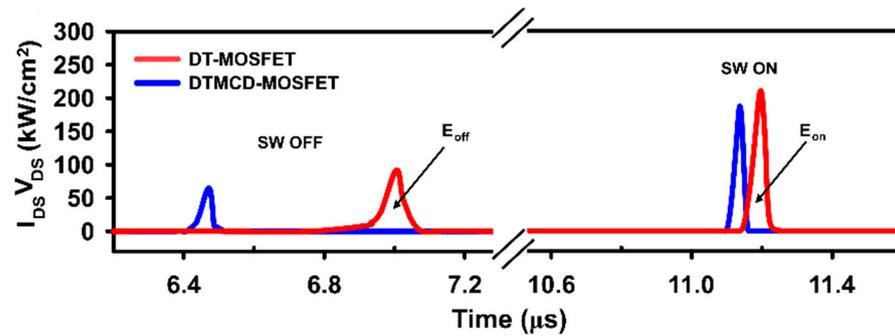
**Figure 13.** Comparison of the power dissipations of DT-MOSFET and DTMCD-MOSFET during the switching transient.
