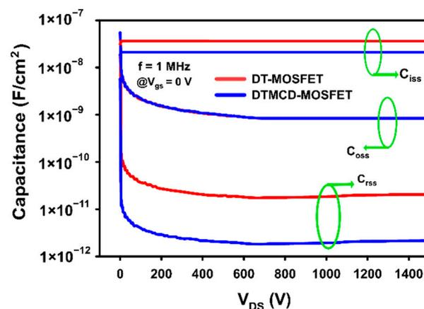
**Figure 11.** Parasitic gate-drain capacitance, input and output capacitance curves of DT-MOSFET and DTMCD-MOSFET with  $V_{GS} = 0 \text{ V}$ .
