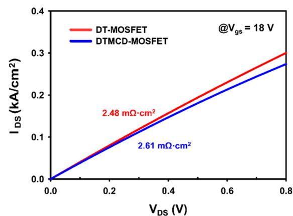
Figure 4. Comparison of the on-state characteristics of DT-MOSFET and proposed DTMCD-MOSFET.
