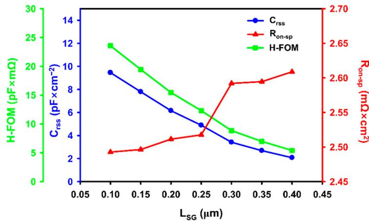
**Figure 2.** Comparisons of the specific on-resistance ( $R_{on-sp}$ ), gate-drain capacitance ( $C_{rss}$ ), and H-FOM characteristics for different  $L_{SG}$  of DTMCD-MOSFET.
