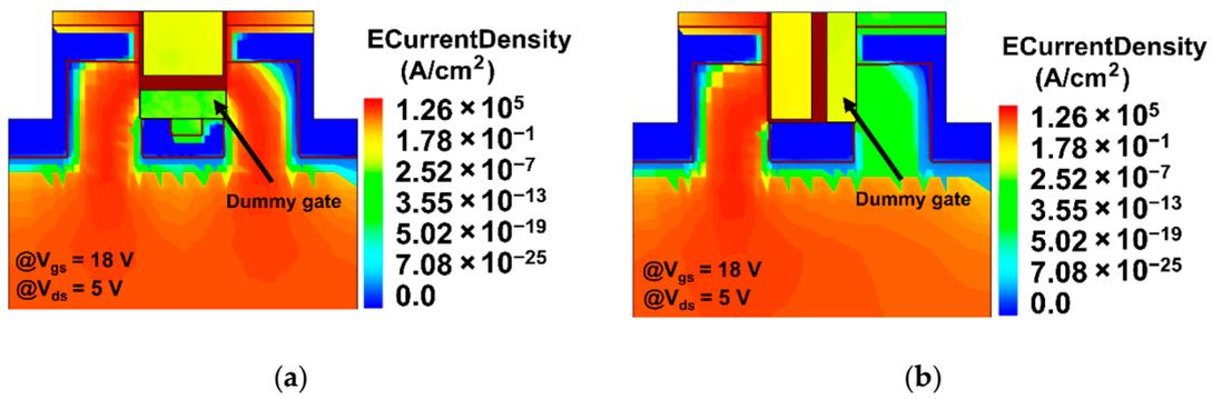
Figure 5. Cross-sectional view of electron current density distribution of (a) proposed DTMCD-MOSFET with horizontally separated gate structure and (b) DTMCD-MOSFET with vertically separated gate structure.
