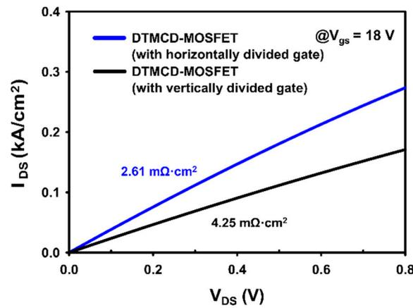
Figure 6. Comparison of the on-state characteristics of two MOSFETs with gate structures separated in horizontal and vertical directions, respectively.
