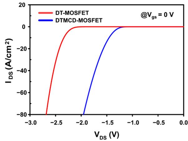
Figure 9. Third quadrant characteristics of DT-MOSFET and DTMCD-MOSFET.
