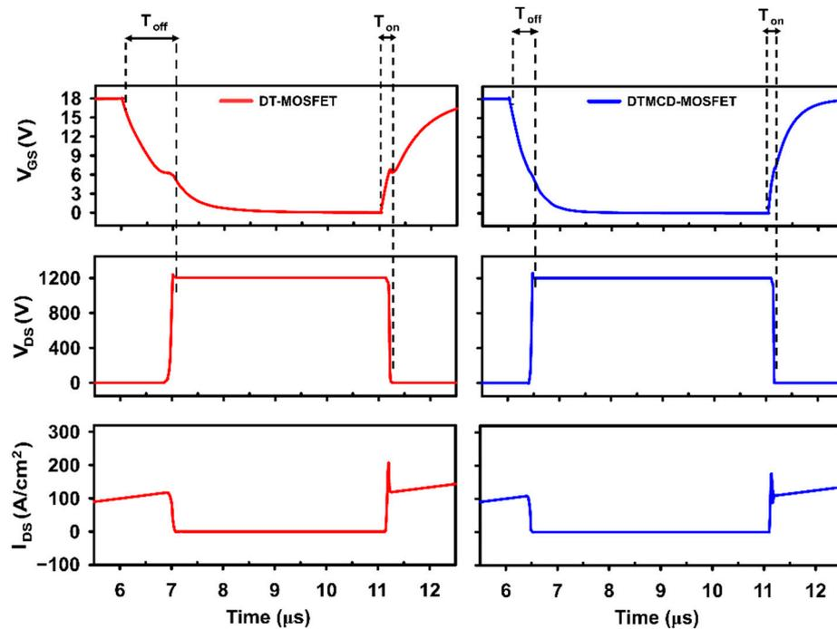
Figure 12. Switching waveforms of DT-MOSFET and DTMCD-MOSFET.
