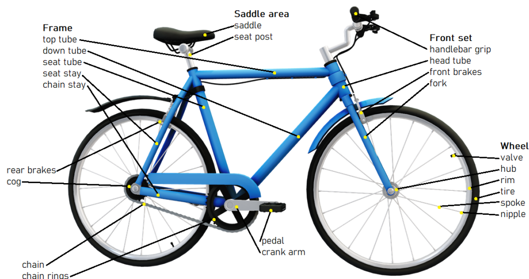
Figure 1. Bicycle parts and their naming conventions [10].
