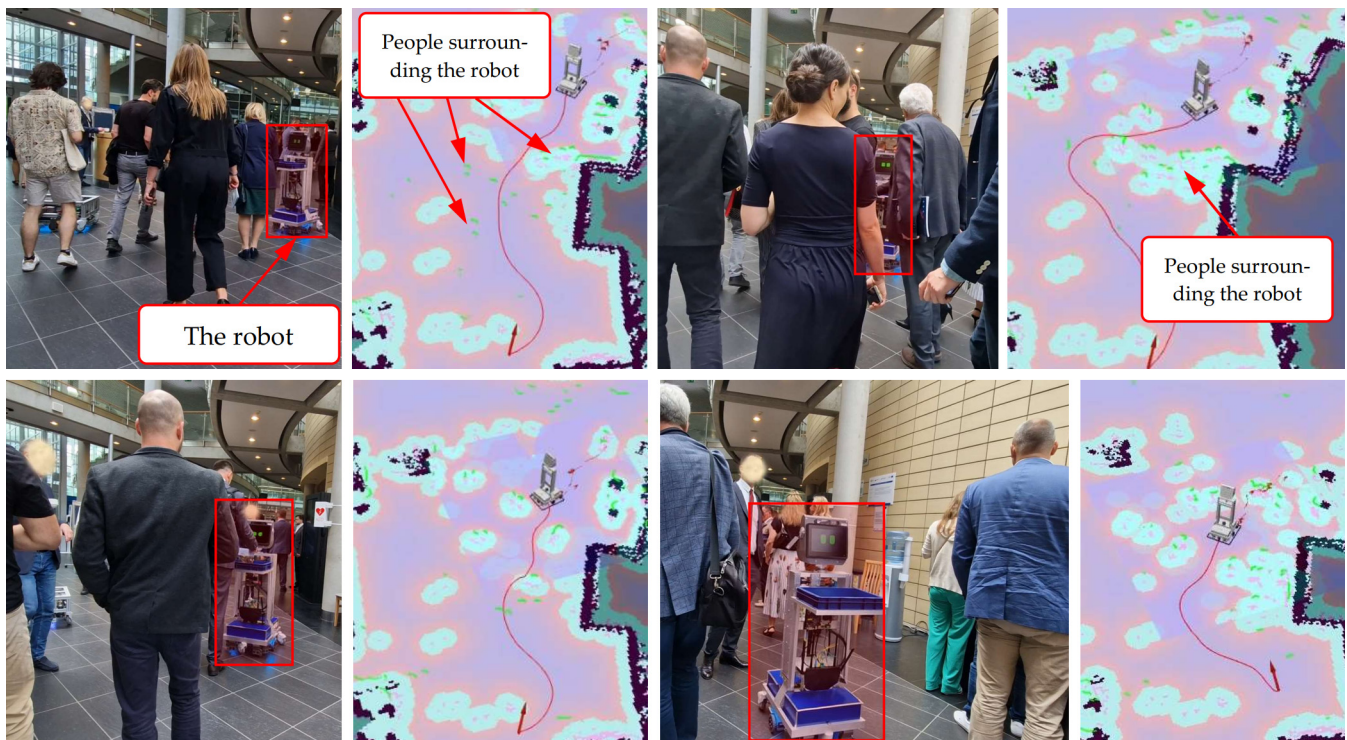
Figure 4. Time-lapse photos showing the various stages of the robot's movement while avoiding humans in a cluttered environment. The robot has been marked in a red frame.
