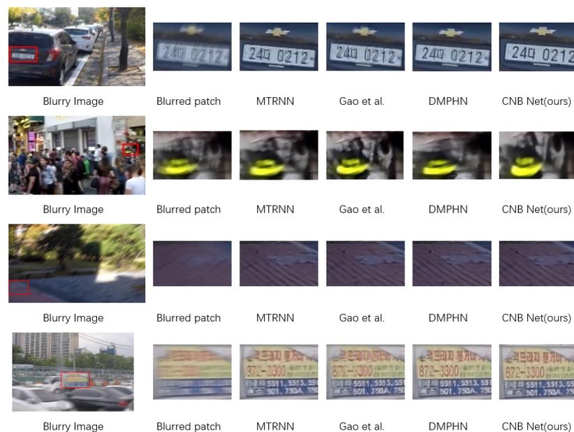
Figure 5. Qualitative comparisons with other methods on the GoPro dataset. The deblurred results listed from left to right are from MT-RNN [22], Gao et al. [20], and DMPHN [23].
