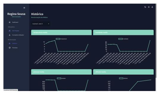
**Figure 3.** History data dashboard based on the selected street. The data are: Temperature, Humidity, Pressure, and Altitude.
