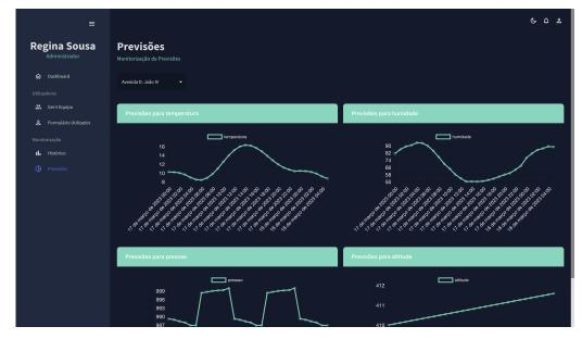
**Figure 4.** Result dashboard for forecasts with prediction for sensors with historical data. The data are: Temperature, Humidity, Pressure, and Altitude.
