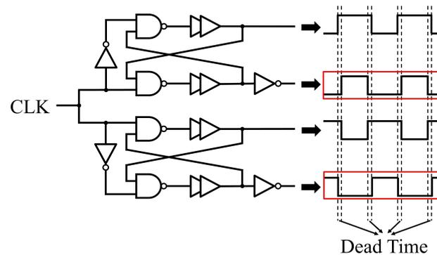
**Figure 5.** Circuit diagram of the dead time generator and its waveform. The waveforms in the red boxes are used to drive the HB driver.
