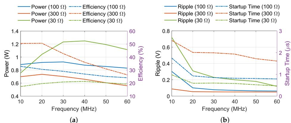
Figure 8. Post-layout simulation result of the charge pump for different loads and different clocks. (a) Output power and efficiency. (b) Ripple and startup time.
