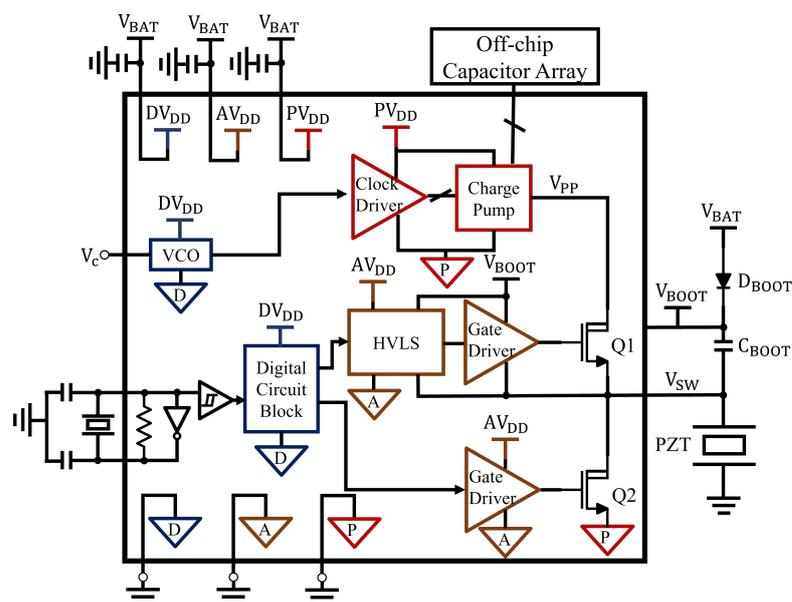
**Figure 2.** System architecture of the proposed ASIC and its periphery components. The blue boxes are digital modules, the brown boxes are analog modules, and the red boxes are power modules.
