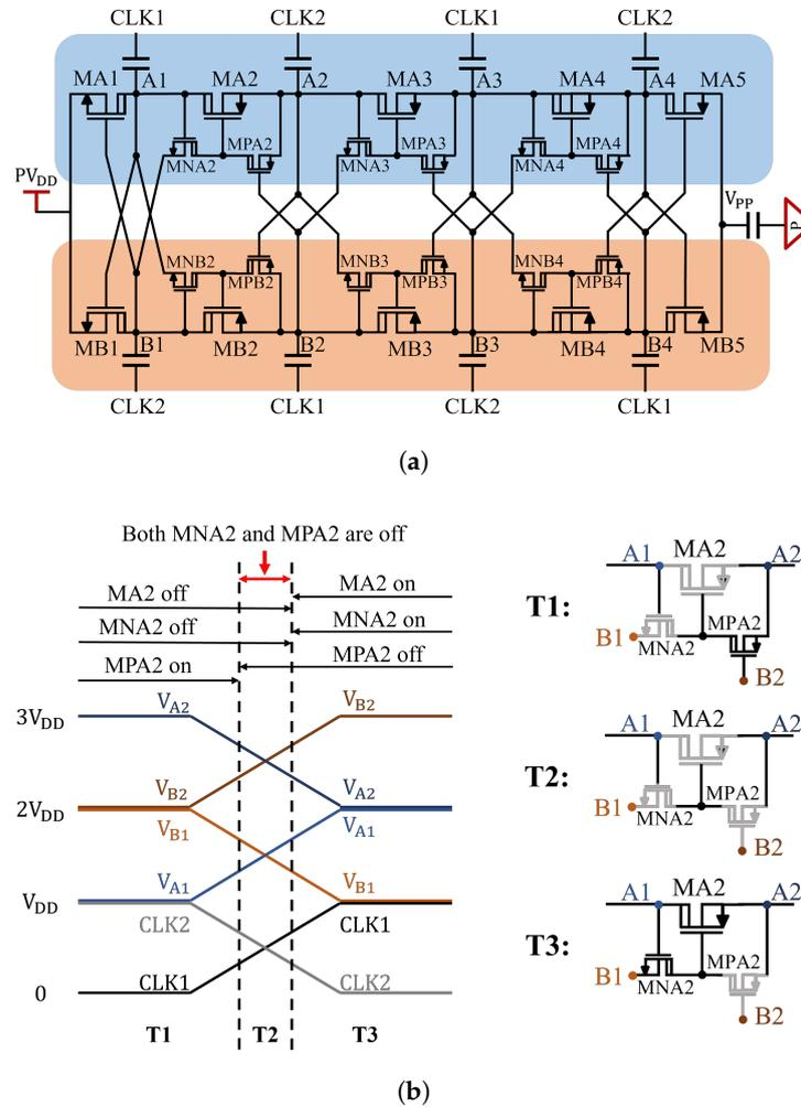
**Figure 3.** (a) Four-stage charge pump in the proposed system (revised from the previous work [24]). (b) Switching waveform and the corresponding operation of a representative CTS MA2.
