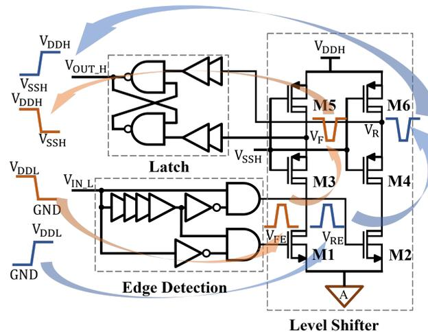
Figure 4. Circuit diagram of the HVLS and its operating principle (revised from the previous work [25]).
