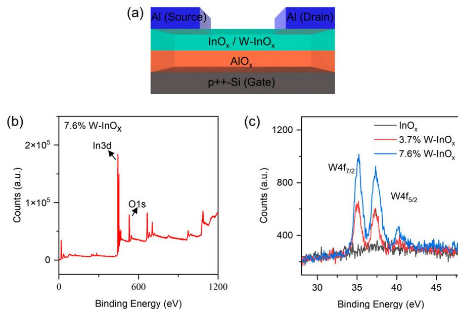
**Figure 1.** (a) Scheme of the electrolyte-gated transistor using the  $\text{AlO}_x$  as an electrolyte layer and the  $\text{W-InO}_x$  as a semiconductor layer. (b) XPS survey for the 7.6%  $\text{W-InO}_x$  film. (c) XPS  $\text{W4f}$  core-level for the  $\text{InO}_x$  films with various tungsten concentrations.
