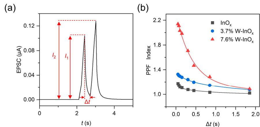
**Figure 3.** (a) EPSCs at  $V_D = 1$  V triggered by a pair of gate voltage pulses;  $I_1$  and  $I_2$  are the current values at the end of the first and the second pulses. The pulse amplitude, width, and period are 2 V, 0.3 s, and 0.6 s, respectively. (b) PPF index as a function of the interval time  $\Delta t$  and fitted by a double-phase exponential function.
