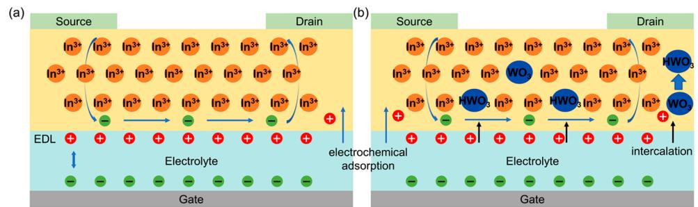
**Figure 4.** (a) Schematic diagram of the EDL and electrochemical adsorption in the InO<sub>x</sub> electrolyte-gated transistor. (b) Schematic diagram of the electrochemical adsorption and ion intercalation in the W-InO<sub>x</sub> electrolyte-gated transistor.
