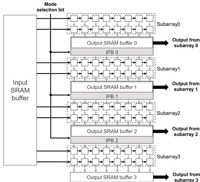
**Figure 4.** The hardware architecture of VerSA. The internal architecture of a single processing element in VerSA is the same as that in the conventional SA. In the case of the dense mode, the hardware performs the operations of Steps ②, ③, and ④, as shown in Figure 2. In the case of the sparse mode, the hardware performs the operations of Steps ②, ④, and ⑤, as shown in Figure 2.
