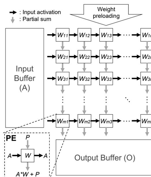
**Figure 1.** The conventional systolic array architecture with weight stationary dataflow. When performing  $A \times B = C$ ,  $A$ ,  $B$ , and  $C$  correspond to the input ( $A$  in the figure), weight ( $W$  in the figure), and output ( $O$  in the figure), respectively.
