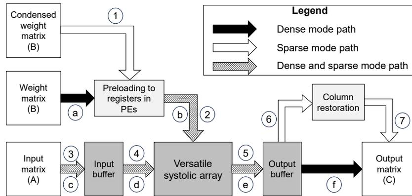
**Figure 2.** The overall execution flow of the VerSA architecture ( $A \times B = C$ ). The steps from ① to ⑦ correspond to sparse mode operations while those from ① to ⑦ correspond to dense mode operations.
