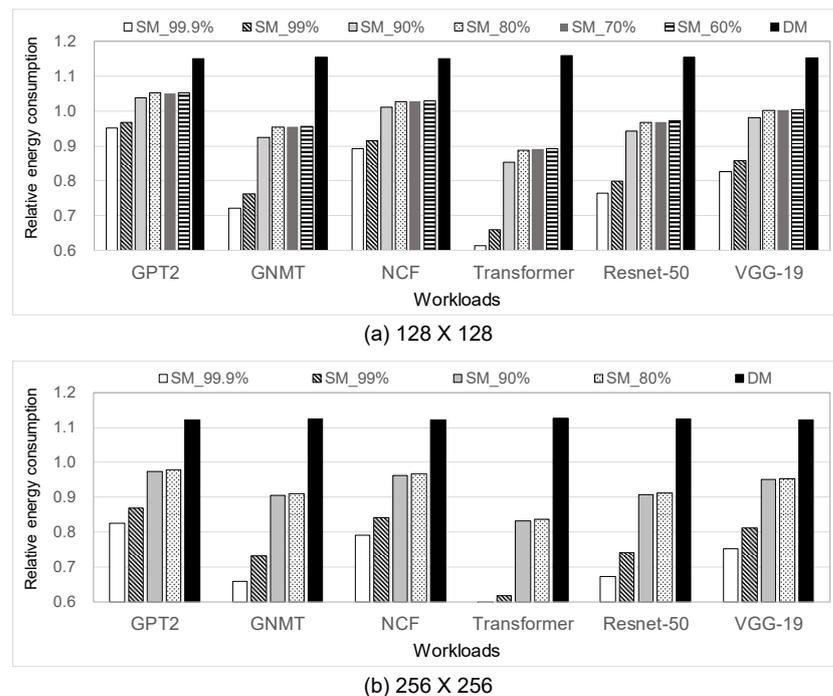
**Figure 9.** The energy consumption of our VerSA normalized to the conventional SA (=1.0). SM\_X% is the sparse mode with an X% sparsity level. DM means the dense mode.
