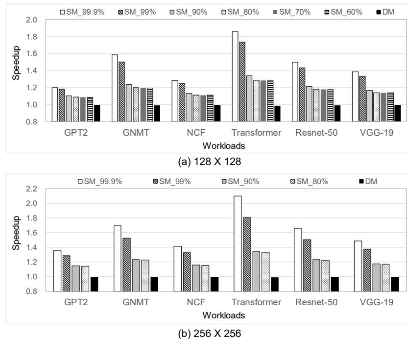
**Figure 8.** The speedup of VerSA architecture when compared to the conventional SA. SM\_X% represents the sparse mode with an X% sparsity level. DM is the dense mode. The  $\text{Num}_{\text{subarray}}$  is set to eight in both  $128 \times 128$  and  $256 \times 256$  SA.
