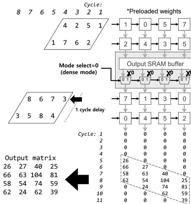
Figure 7. An example of dense mode operations in VerSA.
