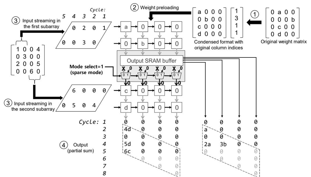
Figure 5. An example of sparse mode operations in VerSA.
