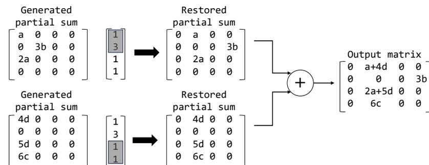
**Figure 6.** The restoration of the partial sum matrices and summation in VerSA, which correspond to the operations of Steps ⑥ and ⑦ in Figure 2.
