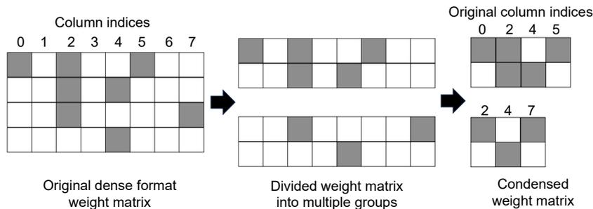
**Figure 3.** An example of a column-wise matrix condensing with a  $4 \times 8$  weight matrix and  $NumRows_{subarray} = 2$ . The gray and white cells represent the non-zero and zero weight elements, respectively.
