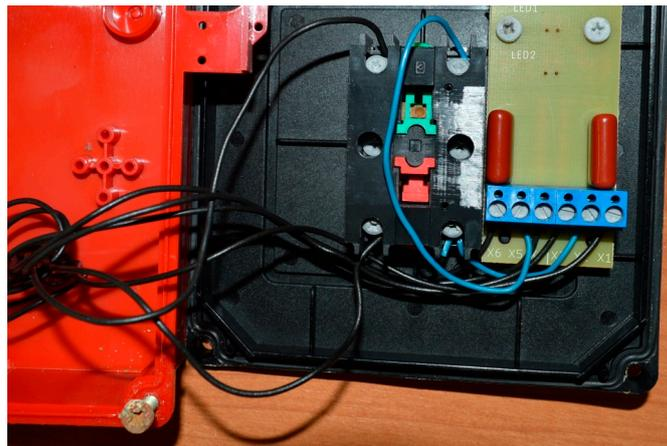
**Figure 18.** A view of an example of a sample of the *FCB activating device* after environmental and EMC testing positive; the actuator worked properly despite visible corrosion marks (on screws and connections).
