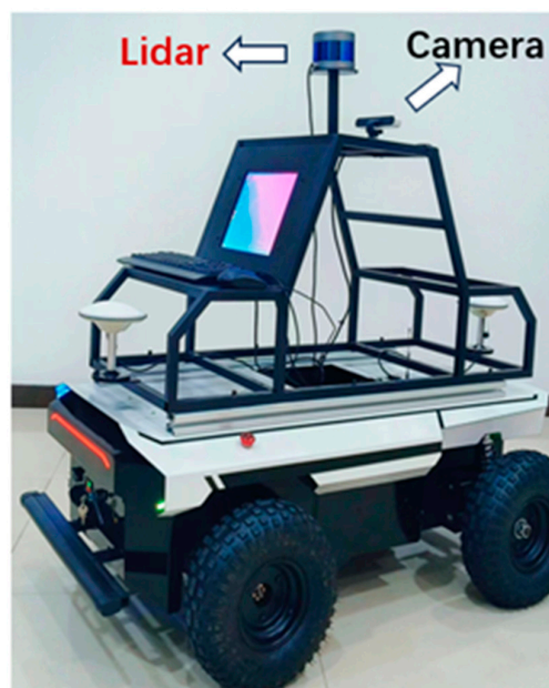
Figure 1. A LiDAR–camera fusion-enabled ground surveillance robot.
