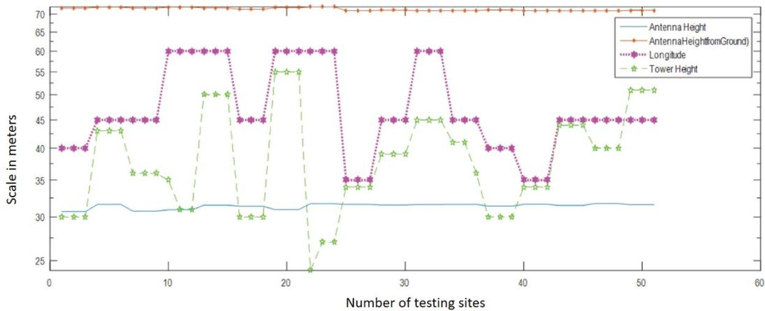
**Figure 4.** Comparative analysis on 15 MHz-bands for 4G technology with antennas height and tower heights in meters, with longitudinal variations for the antennas.
