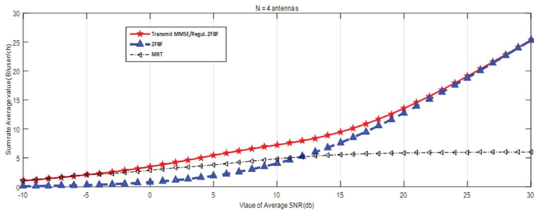
**Figure 1.** Performance of Transmit MMSE, MRT and ZFBF is low for less antennas  $N$  ( $N = 4$ ) and user function SNR, (signal to noise ratio received at the user end) shows that high SNR limit the interuser interface and transmit MMSE performs best.
