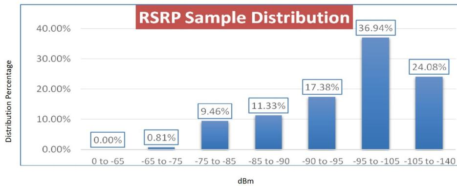
**Figure 6.** The reference signal received power (RSRP) efficiency for our tested scenarios distribution percentage.
