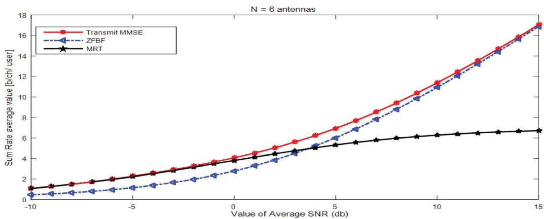
**Figure 2.** Performance of Transmit MMSE, MRT and ZFBF increase with antennas  $N$  ( $N = 6$ ), with ZFBF and MRT compensate against average SNR and user function SNR (signal to noise ratio received at the user end) shows that high SNR limit the interuser interface and transmit MMSE performs best.
