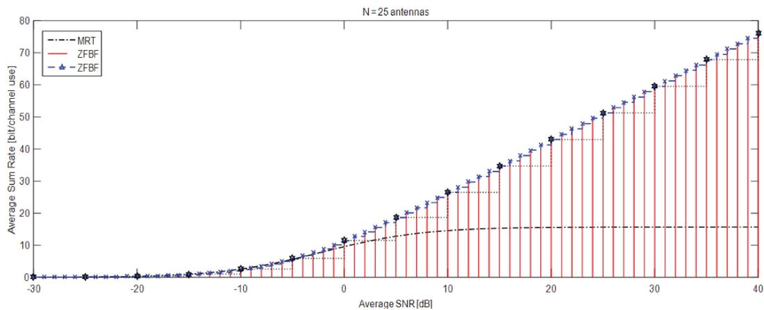
**Figure 3.** Performance of Transmit MMSE, MRT and ZFBF with antennas  $N = 25$ . ZFBF and MRT compensate against average SNR and user function SNR shows that high SNR limit the interuser interface and ZFBF compensate with transmit MMSE and increase with densification of network antennas.
