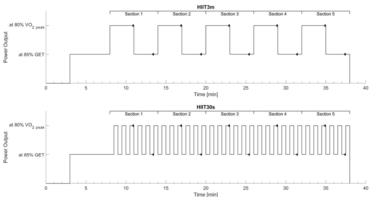
**Figure 1.** Scheme of HIIT3m and HIIT30s protocol regarding interval intensities and duration. The black squares demonstrate the 10 s period, where the means for work (loaded) and resting (unloaded) phases were calculated.
