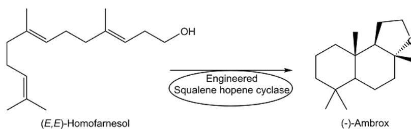
**Figure 8.** Enzymatic process for the industrial production of the fragrance ingredient (-)-Ambrox.
