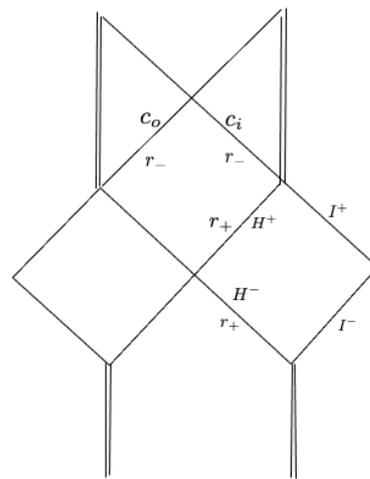
**Figure 3.** Penrose diagram of the maximal analytic extension of the RN metric.  $H^+$  is the future event horizon,  $H^-$  the past one;  $c_o$  and  $c_i$  are, respectively, the outgoing and ingoing sheets of the Cauchy horizon located at  $r_-$ .
