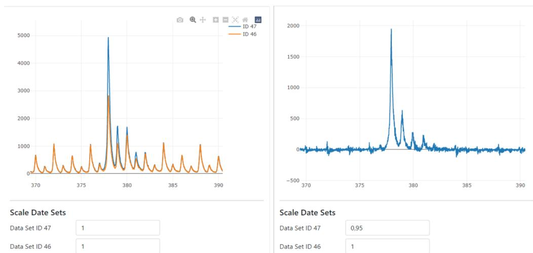
**Figure 2.** Detailed view of the data representation. Left: comparison of two mass spectra plotted on top of each other with a linear y-axis. Right: difference between the same two mass spectra, with a scaling factor of 0.95 applied to the first mass spectrum.
