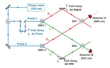
**Figure 1.** Two-photon interference setup with two synchronously-pumped spontaneous parametric down-conversion (SPDC) crystals BBO1 and BBO2. The rate of counting signal and idler photons in coincidence at Detectors A and B is measured as a function of the path delay of the pump field. The pump intensity is sufficiently weak such that with high probability, only one signal-idler photon pair is present during a measuring period. BS, beam splitter.
