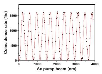
**Figure 4.** Second-order interference of the single signal photons from crystals BBO1 or BBO2 at Detector A in coincidence with the single idler photons from crystals BBO1 or BBO2 at Detector B, as a function of Pump 1 path delay for BBO1 (see Figure 1).
