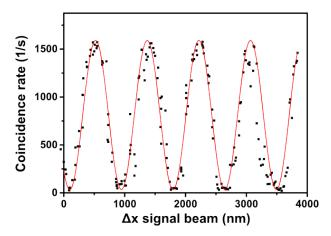
**Figure 3.** Counting rate for single signal photons at Detector A in coincidence with single idler photons at Detector B as a function of the signal path delay as in Figure 2, but with higher resolution.
