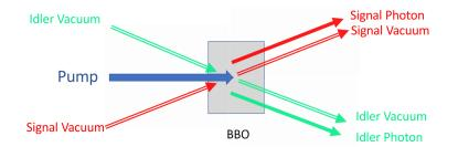
**Figure 5.** Signal- (idler-) photons are created by the mixing in the BBO crystal of the pump field with the vacuum field in the idler (signal) mode, as described by Equations (2) and (3). The signal (idler) field emerging from the crystal is the sum of the vacuum field in the signal (idler) mode and the signal (idler) field resulting from the nonlinear mixing process described by the Hamiltonian (1).
