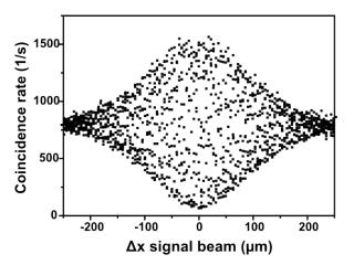
**Figure 2.** Counting rate for single signal photons at Detector A in coincidence with single idler photons at Detector B as a function of the signal path delay (see Figure 1).
