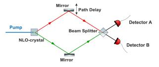
**Figure 6.** Hong–Ou–Mandel setup for observation of a dip in the signal-idler photon coincidence rate at Detectors A and B. The signal and idler fields, which are assumed here to have the same frequency and polarization, are reflected by the upper and lower mirrors, respectively and can either be reflected or transmitted by the beam splitter (BS).
