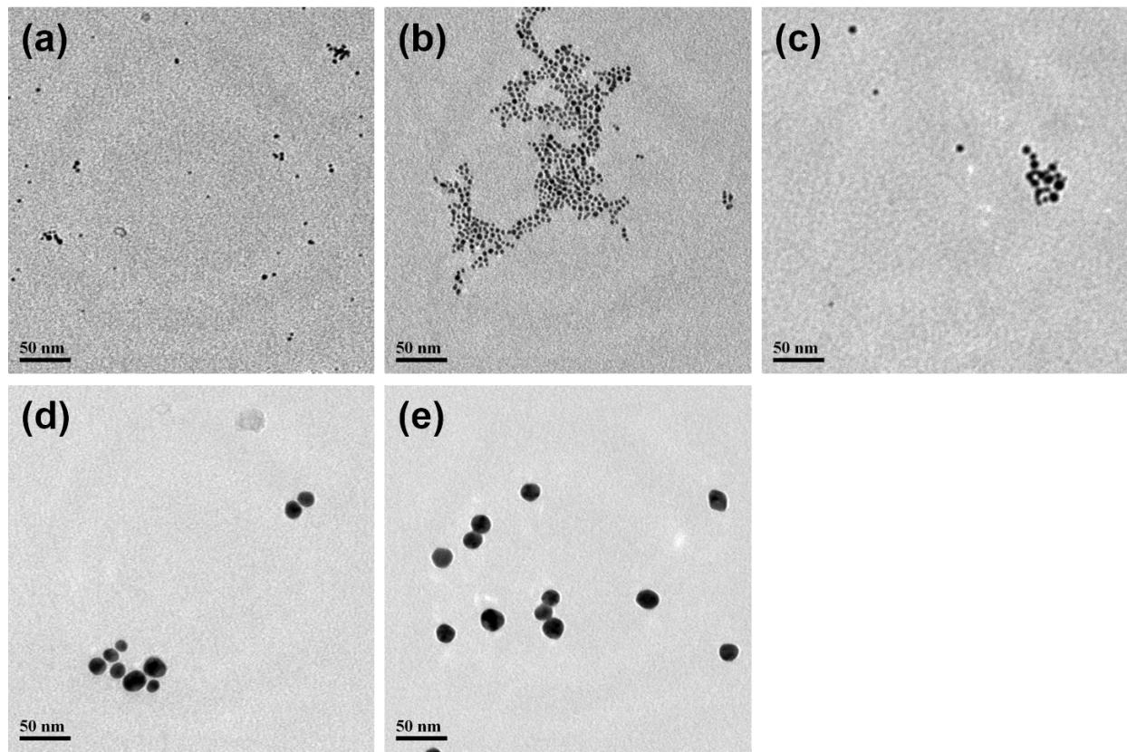
**Figure S1.** TEM images of the produced GNPs (before PDT cross-linking): (a) 2.6 nm; (b) 8 nm; (c) 13 nm; (d) 25 nm; (e) 38 nm.
