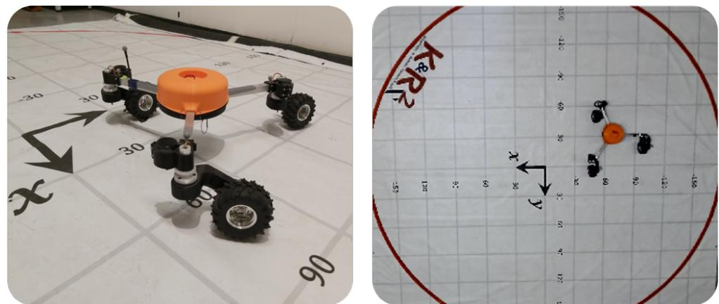
**Figure 4.** On the (left): The COR that was fabricated in the robotic research laboratory. The platform radius ( $r_i$ ) is 0.31 m and the caster wheel arm ( $d_i$ ) is 112.5 m. (right): A camera top view of the experiment arena. A set of 18 *Optitrack Flex-13* cameras for detecting the COR position and orientation were used in order to evaluate the mechanism's performance. The available accuracy is less than one mm in the position and rotational error less than  $0.05^\circ$  of a rigid body.
