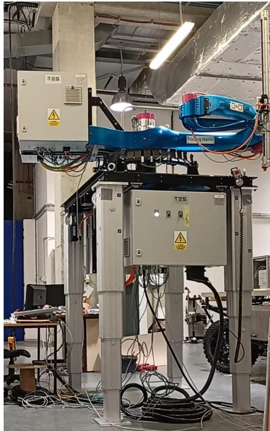
**Figure 13.** Lifting the robotic base of the experimental printing robot (see video in [44]).
