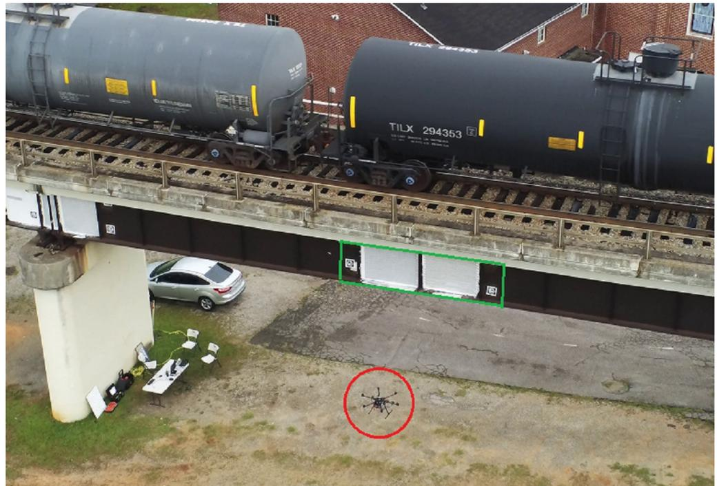
**Figure 10.** The UAS used for field deployments during a railroad bridge inspection. The UAS is highlighted with a red circle, and the inspection area is highlighted with a green box.
