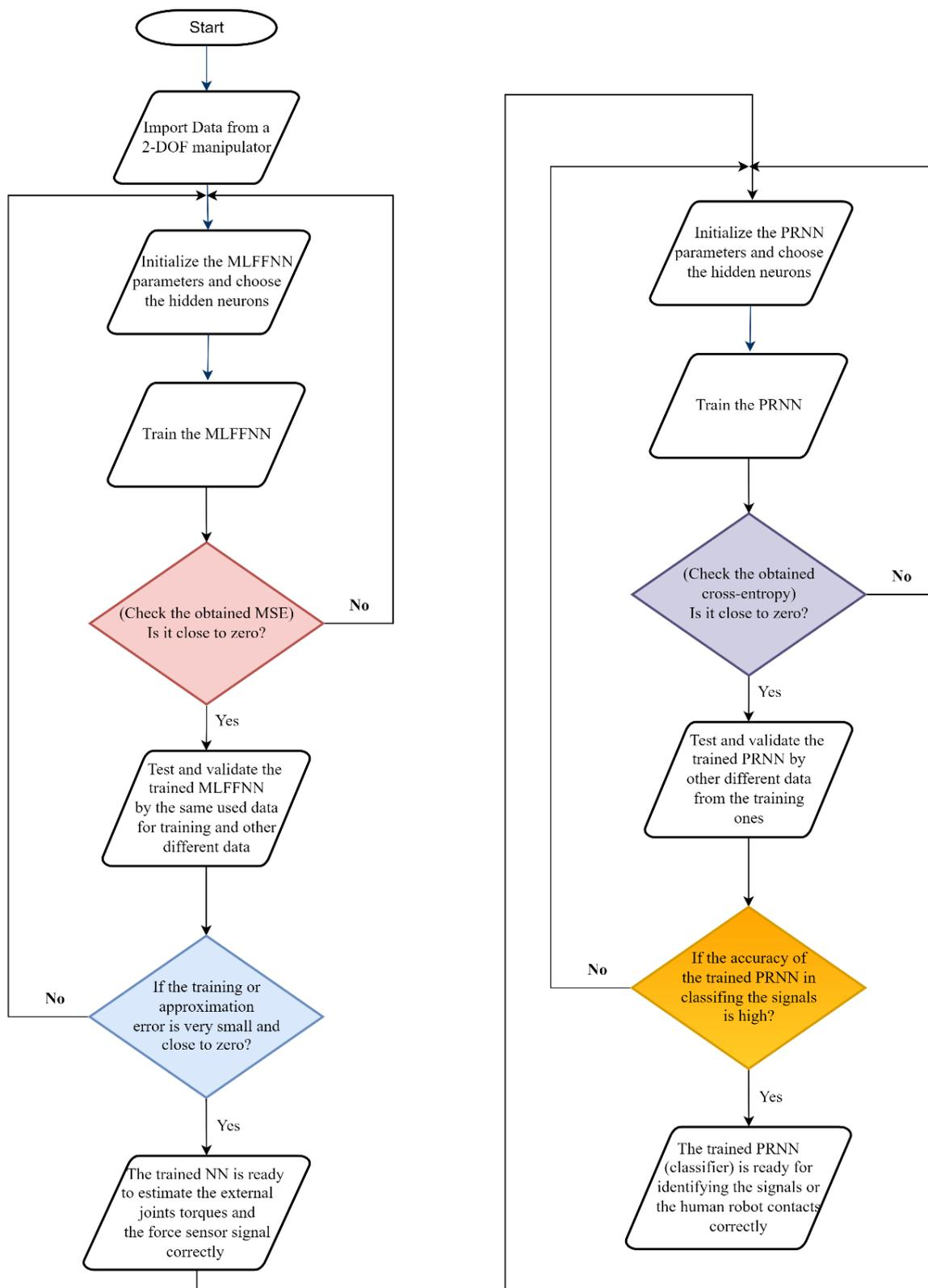
**Figure 4.** The steps followed in the current work start from collecting the data and until readiness for classifying the force sensor signals.
