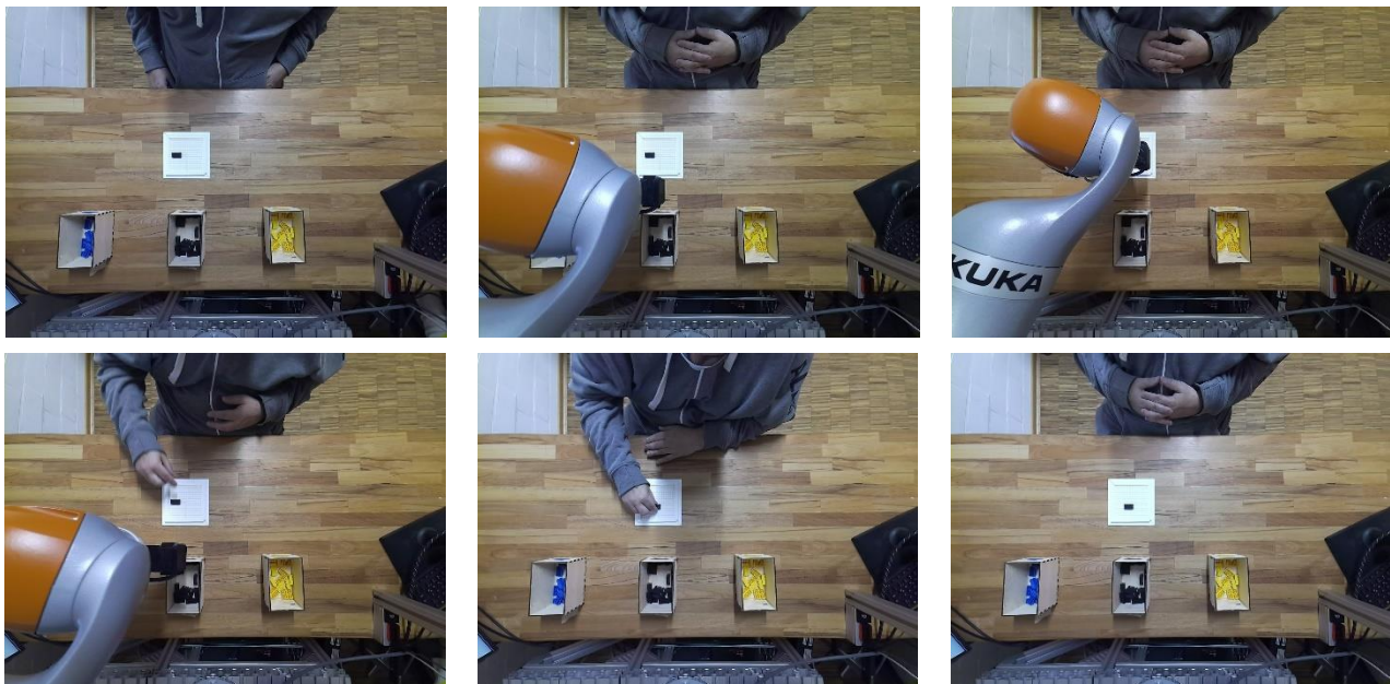
Figure 10. Sequence of the successful interpretation of assistance 6 by the participant. Initially, the brick was placed incorrectly. As a result, the robot performs assistance. After executing assistance 6, the participant reacts and corrects the position of the brick.
