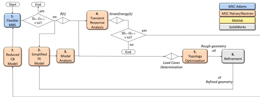
Figure 4. QSL method employed in the work.
