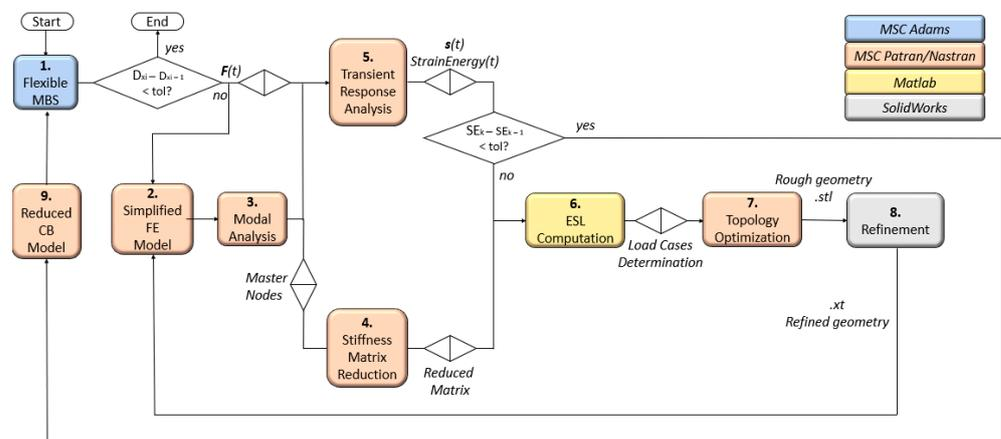
Figure 3. ESL method employed in the work.
