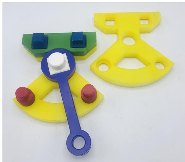
**Figure 3.** Partly finished assembly of the Cranfield Benchmark Problem used in the experiments.
