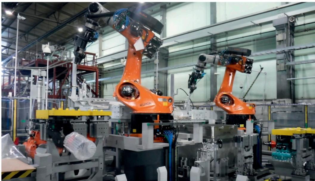
**Figure 1.** Box Encapsulation Plant (BEP) robot rig trial being carried out at National Nuclear Laboratory (NNL)'s rig hall in Workington, Cumbria, UK.
