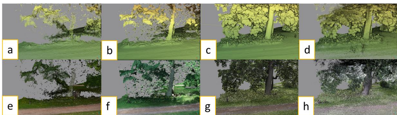
Figure 10. Comparison of point clouds for natural ground vegetation. In the top row, the point clouds are colored with the height ramp, and in the bottom row with RGB colorization.
