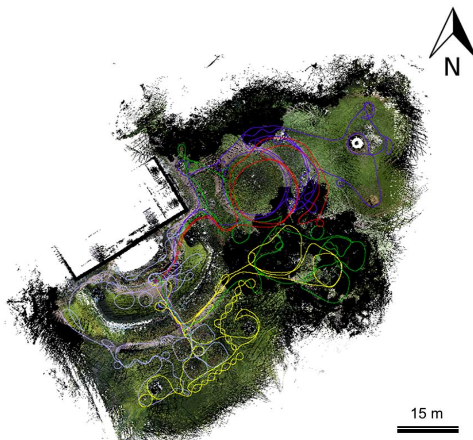
Figure 4. GeoSLAM ZEB Revo RT point cloud with independent measurement trajectories which are colored individually as blue, red, yellow, green, and purple. The point cloud is colored with the data of the integrated camera system, and the black points are laser scanning points that do not have any color value from camera data.
