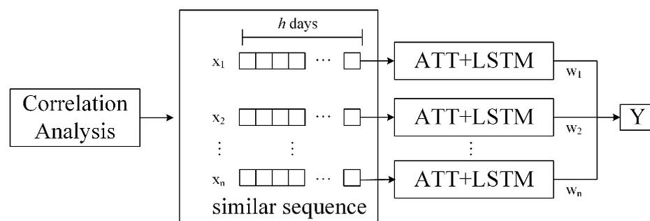
Figure 4. The ATT-LSTM prediction model that considers the synergy of similar time series.
