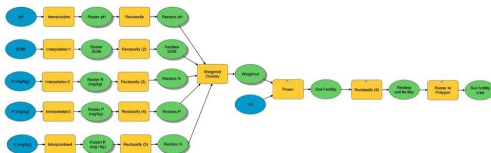
**Figure 8.** Flow chart devised in this study to model SFC.
