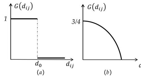
**Figure 5.** Attenuation function of 2SFCA (a) and kernel density 2SFCA (b).
