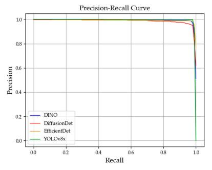
Figure 8. PR curves for four object detection models.
