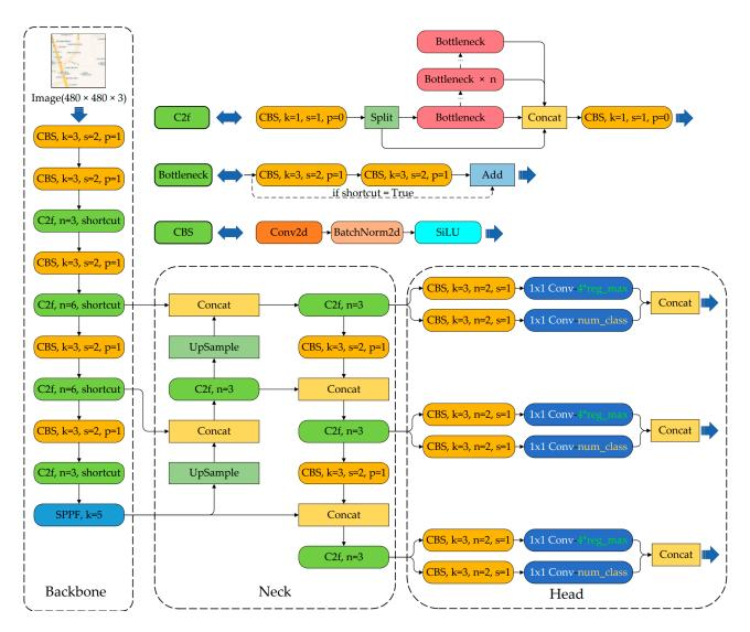
**Figure 5.** Schematic of the YOLOv8 model structure. (This paper uses Amap as an example, in which the Chinese characters do not affect the experimental results).
