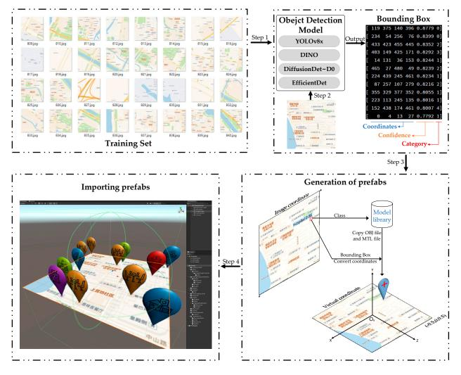
**Figure 6.** Schematic of the automated method for generating prefabs of AR map point symbols. (This paper uses Amap as an example, in which the Chinese characters do not affect the experimental results).
