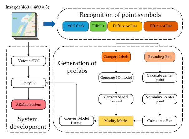
**Figure 2.** The framework of generating AR map point symbol prefabs based on object detection model. (This paper uses Amap as an example, in which the Chinese characters do not affect the experimental results).
