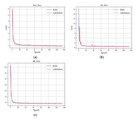
Figure 10. Loss curves of YOLOv8x. (a) box\_loss; (b) cls\_loss; (c) dfl\_loss.
