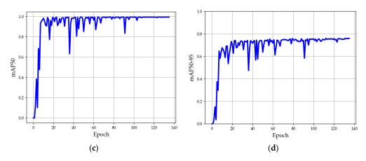
Figure 9. Training process of YOLOv8x. (a) Precision; (b) recall; (c) mAP<sub>50</sub>; (d) mAP<sub>50-95</sub>.
