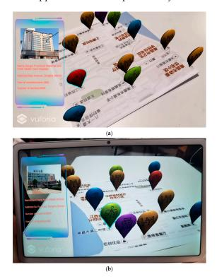
**Figure 12.** Visualization of the running effects of the AR prototype system developed in this paper. (a) A screenshot of the AR map prototype system in operation. (b) A photo of the AR map prototype system running on the validation device. (This paper uses Amap as an example, in which the Chinese characters do not affect the experimental results).
