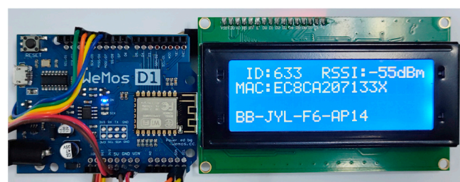
Figure 1. The AP scanner based on ESP8266 microcontroller displaying the MAC address, name, and received signal strength indicator (RSSI) of an AP installed in our lab.
