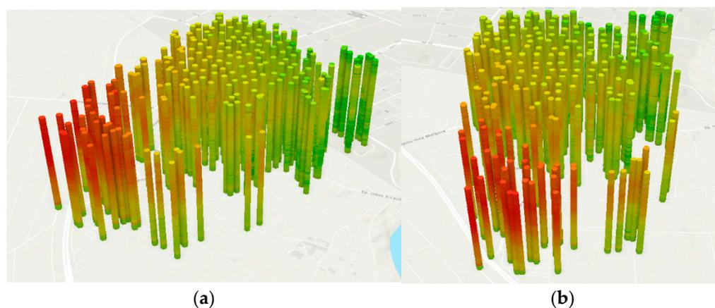
**Figure 11.** A presentation of 3D visualization of PSI time series displacement values in Sindos Region from 2015 to 2020. The value for each date is presented as a tile in space. The orientation of image (a) is SE to NW, while that of image (b) is SN.
