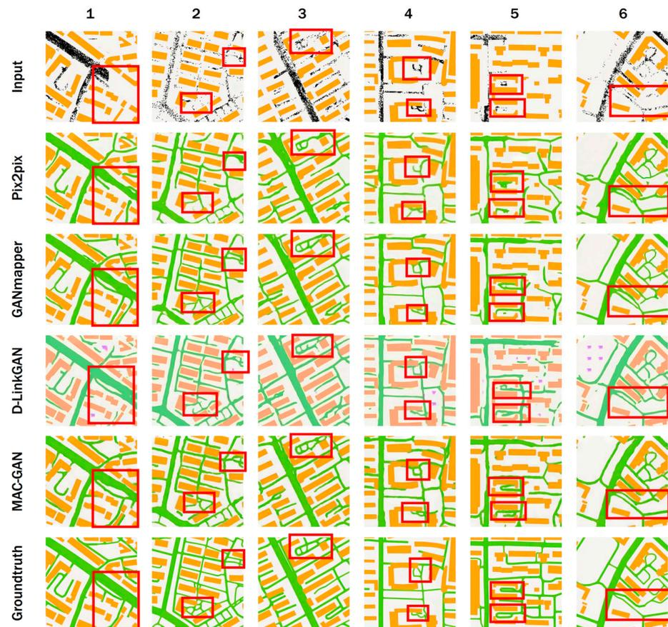
**Figure 9.** Results of MAC-GAN, Pix2pix, GANmapper, and DLink-GAN. Columns 1–6 in Figure 9 represent the six different study areas. In order, the six rows of images in columns 1–6 are the input, the generated results of the four models, and the ground truth. The area marked with a red box is the complex area with sparse or missing trajectories.
