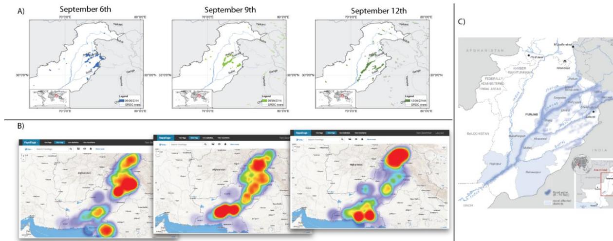
**Figure 2.** Affected flood areas as derived from different sources: (A) flood signal from GFDS for 6, 9 and 12 September. (B) heat map based on flood related Twitter activity for 6, 9 and 12 September; and (C) inundation map published by UN-OCHA in October 2014, outlining all areas that were inundated at some point in September 2014
