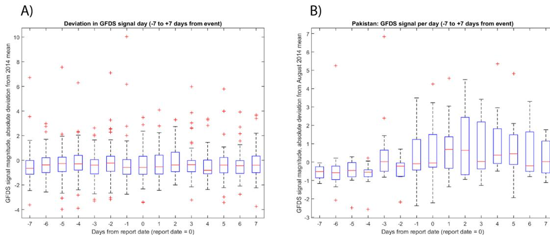
**Figure 4.** Box plots showing the distribution of signal deviation from the mean, for (A) all 80 flood events (*i.e.*, 80 locations) reported throughout 2014 in the Philippines; and (B) the September 2014 floods in Pakistan at 17 locations. For the event date (“day 0” on x-axis), we used the specific reported event date for each individual event for the Philippines; and 4 September 2014 for Pakistan.
