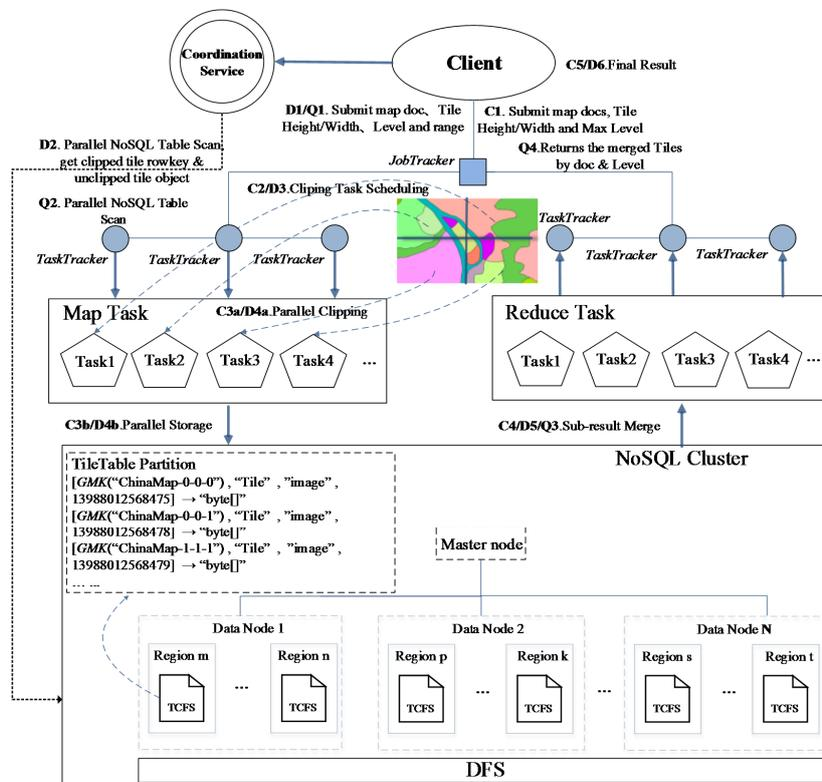
Figure 9. MapReduce-based tile map parallel processing framework.
