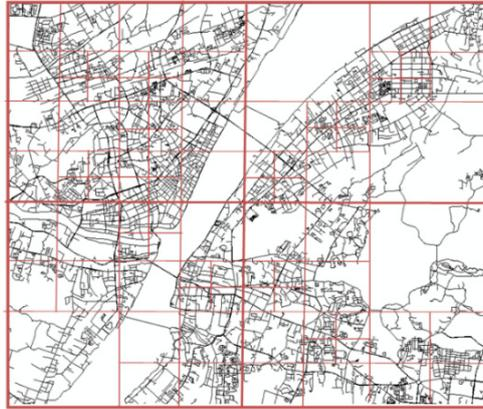
Figure 11. Quadtree-based partition graph of a vector map in dynamic tile clipping.
