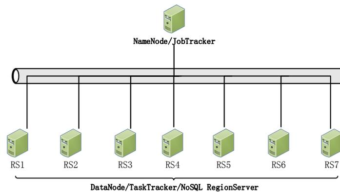
Figure 14. NoSQL cluster-based tile processing architecture.
