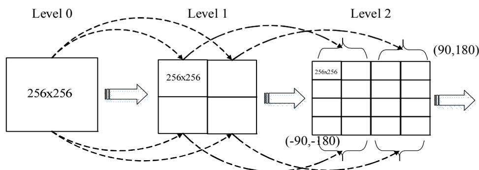
Figure 2. Quadtree-based tile-clipping pattern for global map tile generation.
