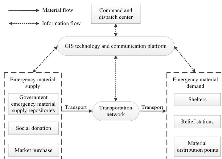
Figure 1. The flow chart of emergency material vehicle dispatching and routing
