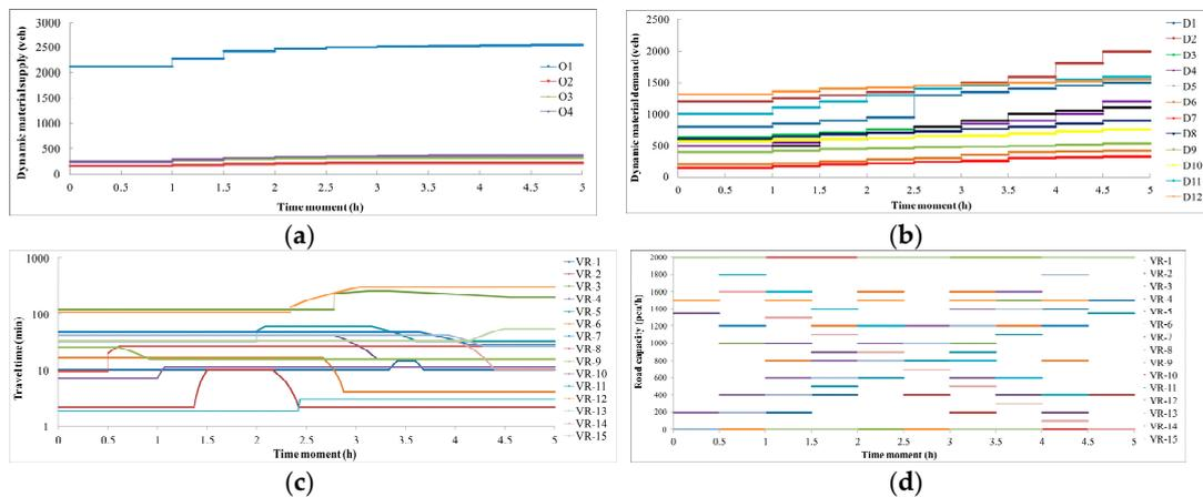
Figure 7. The dynamic environment variable: (a) the dynamic emergency material supply of emergency material depositories without exportation; (b) the dynamic limited emergency material demands of disaster points without importation; (c) the dynamic travel times of vulnerable roads; (d) the dynamic capacity of vulnerable roads, where “pcu” means “passenger car unit” and “pcu/h” refers to the number of vehicles passing through road per hour.
