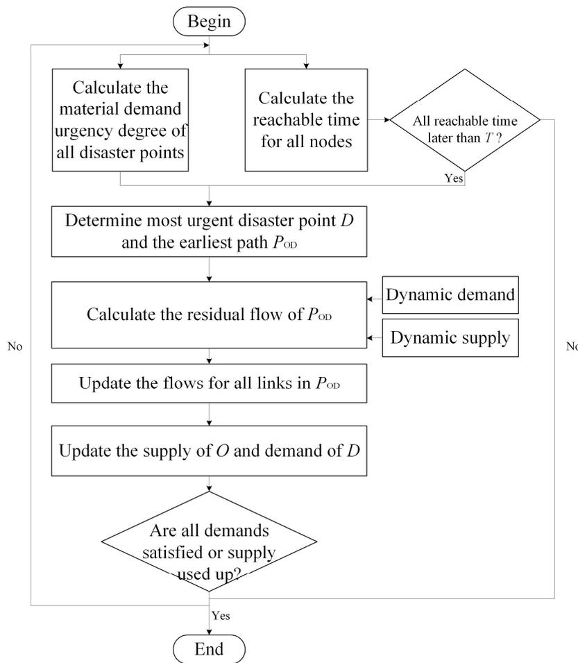
Figure 4. The flowchart of the solving method.
