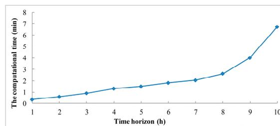
Figure 14. The time performance of the continuous-time dynamic network flow algorithm in solving the EMVDR problem.
