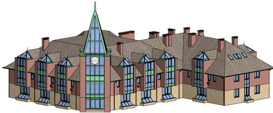
**Figure 1.** 3D model of the city hall, located within the studied area, modelled based on the data from terrestrial laser scanning. Source: own work.
