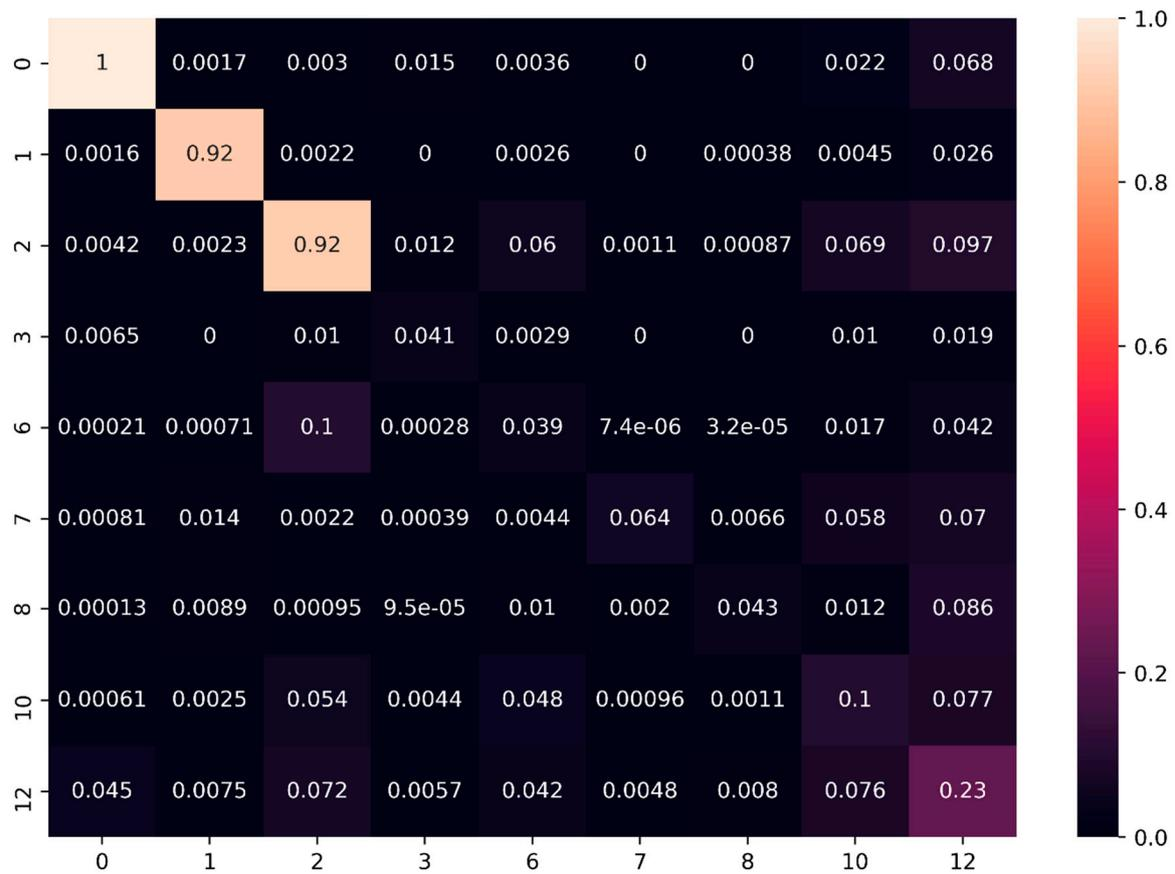
**Figure 17.** Normalized Confusion matrix of our semantic segmentation approach over the full S3DIS dataset.
