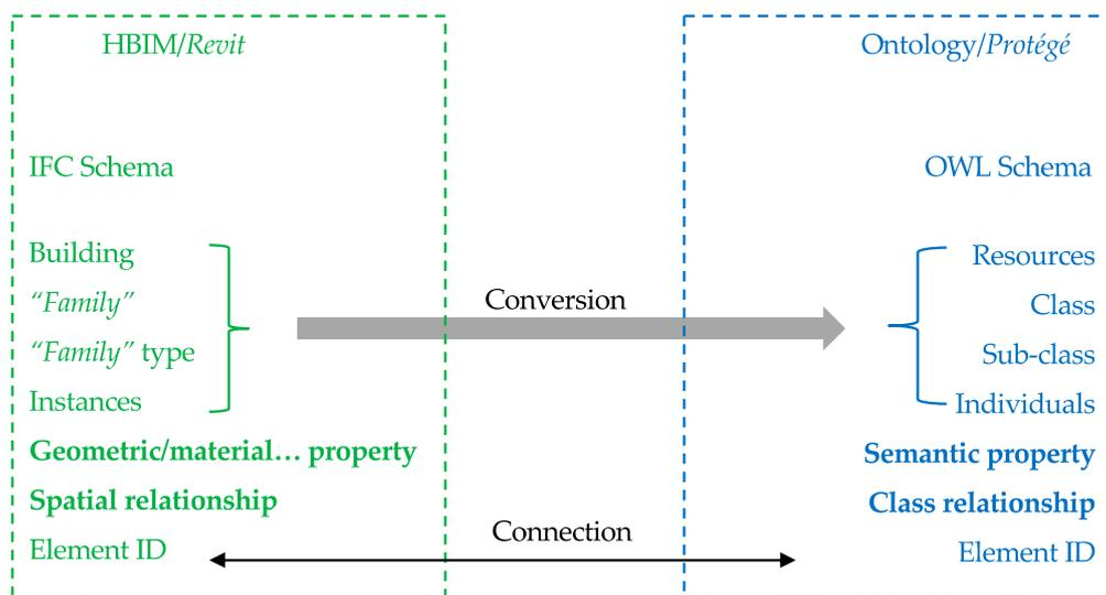
**Figure 6.** The correspondence between HBIM and ontology.
