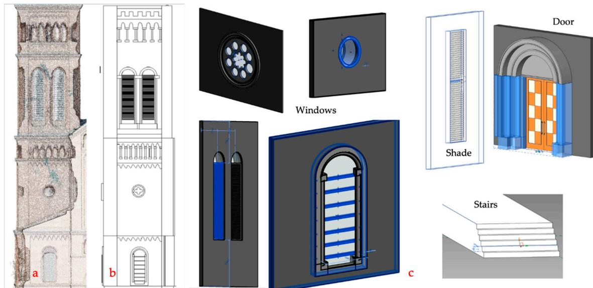
**Figure 3.** (a) The point clouds imported in BIM platform, (b) the HBIM structures created by reverse design, and (c) some typical “classes” composing the church on the reference of the point cloud
