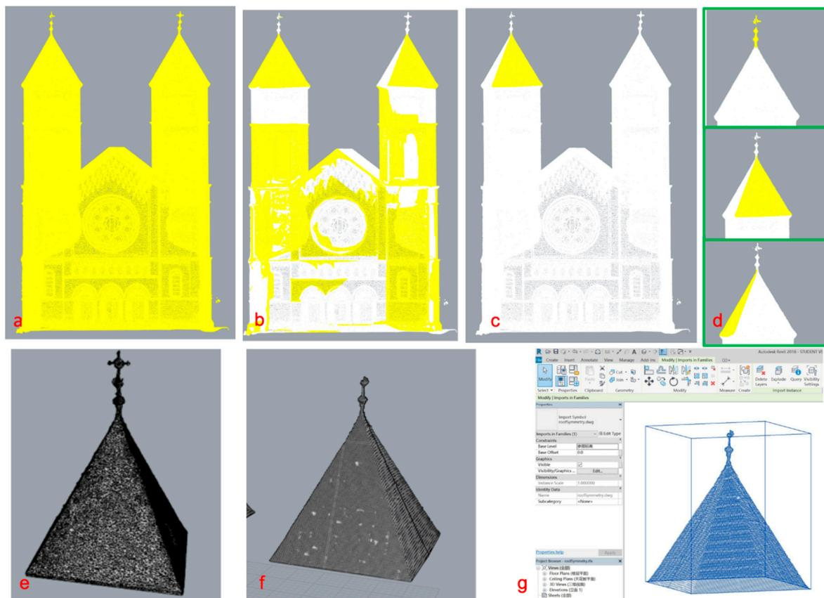
**Figure 4.** The explosion processing to segment the holistic mesh (a) into small blocks by a multi-layered explosion (b,c). The primitive representing the church’s primary component is then generated based on the merging of several small blocks (d). The surface mesh (e) is converted to NURBS curve based solid geometry by adding thickness (f) and translated in a BIM environment (g).
