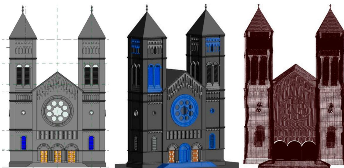
**Figure 10.** The final HBIM models in 2D and 3D views using manual scan-to-HBIM (left and middle) and semi-automated mesh-to-HBIM (right).
