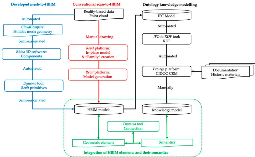
**Figure 1.** Workflows of the HBIM modeling and the integration with ontological knowledge.
