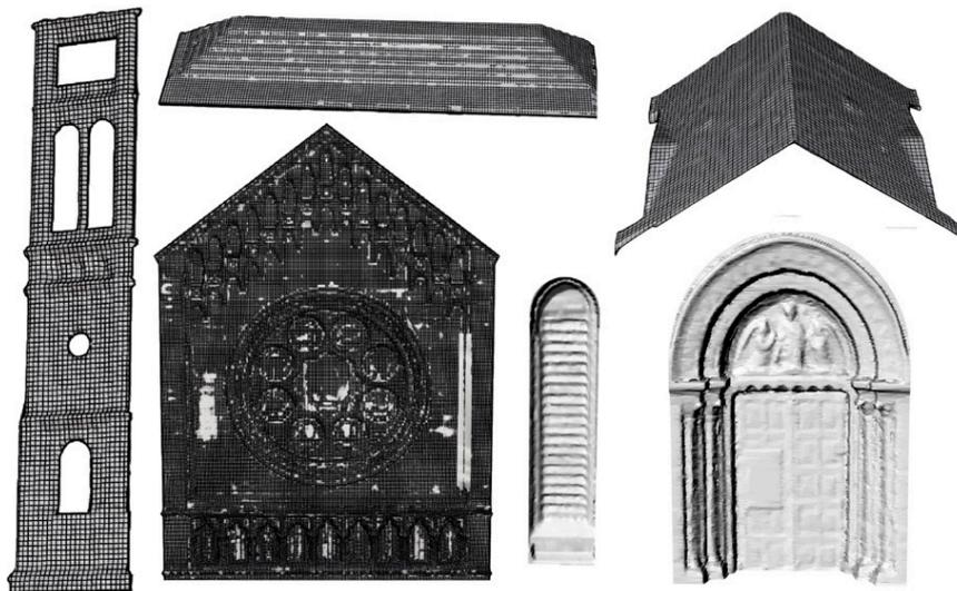
**Figure 5.** The segmentation, combination and extrusion process to transfer the holistic surface mesh into individual solid elements
