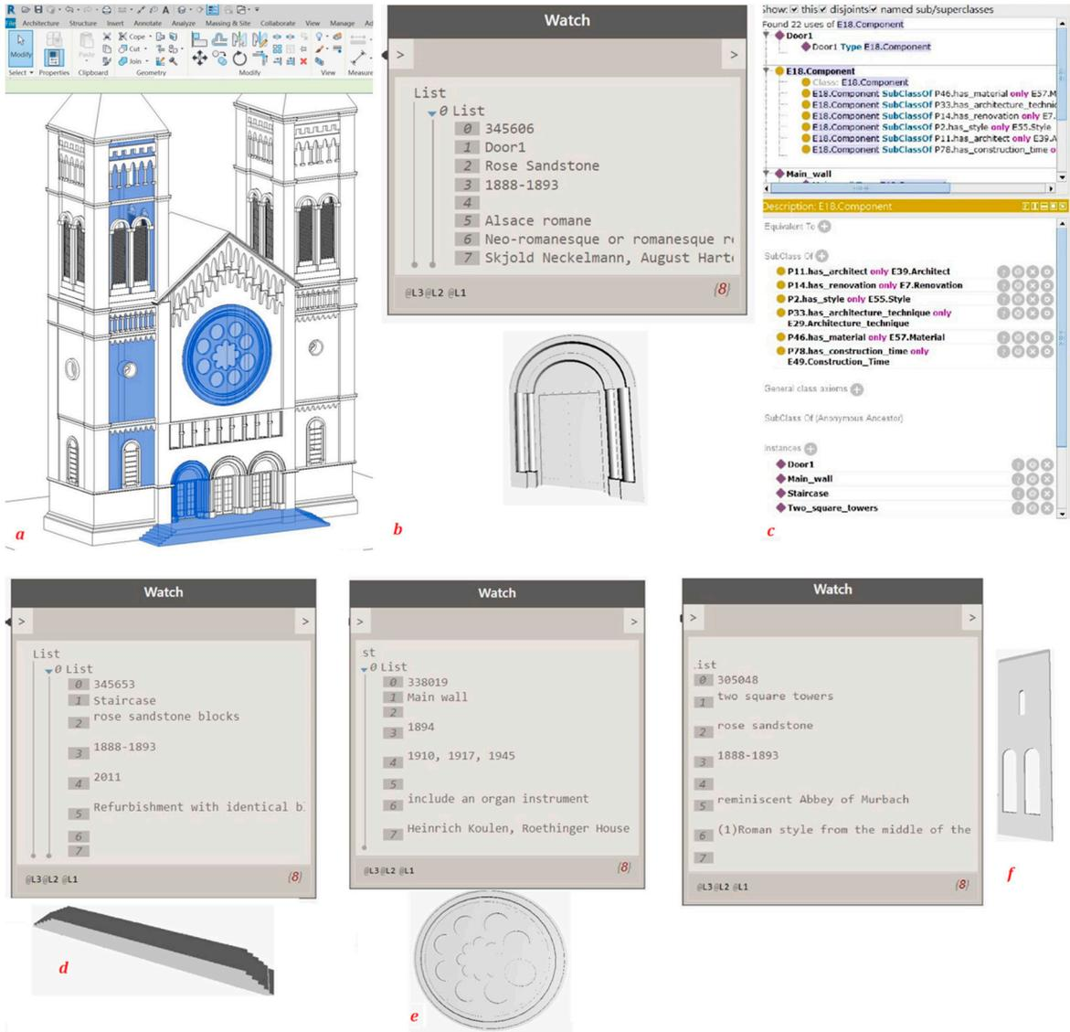
**Figure 11.** The browsing result of some heritage components in *Dynamo* with geometry and knowledge. The “watch” window (b, d, e, f) in the *Dynamo* interface can display the knowledge of selected element of HBIM model (a) in the *Revit* platform. The knowledge in “watch” window derives from previously defined knowledge model (c).
