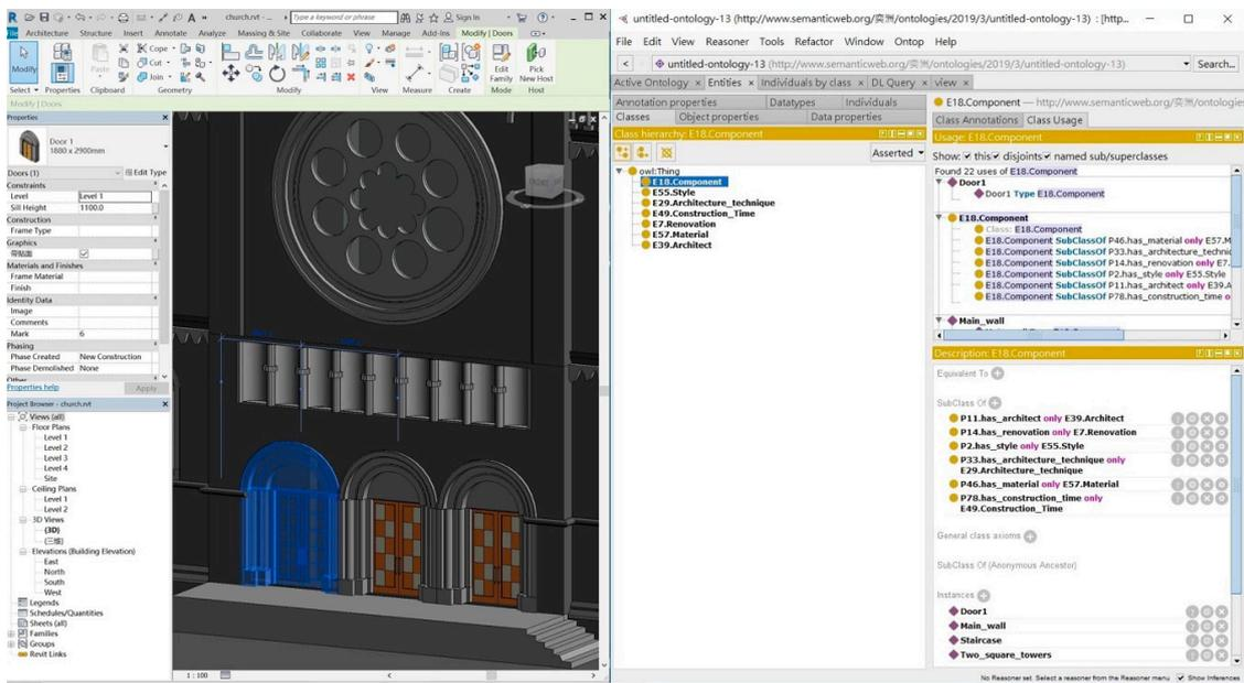
Figure 7. Ontological knowledge modeling for the HBIM entities within the standards of CIDOC CRM.
