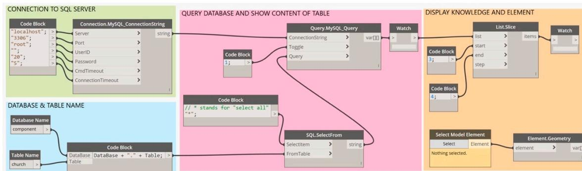
**Figure 9.** The connection of HBIM elements and ontological knowledge based on *Revit Dynamo*, where the corresponding knowledge of the element selected in *Revit* can be displayed in the “watch” window.
