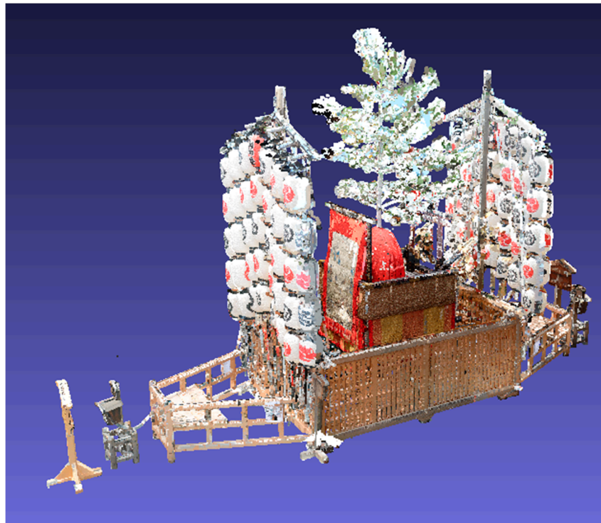
Figure A2. Laser-scanned point cloud of the Hachiman-Yama float ( 2.62 \times 10^7 points).
