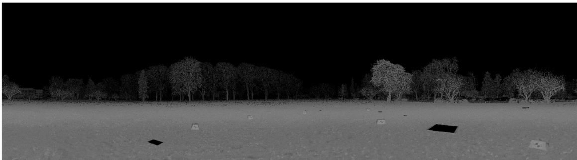
**Figure 4.** Example of a TLS 2D panoramic image, colored by intensity (grayscale). Black pixels indicate no laser pulse returns and are present in locations with standing water (specular reflection), regions with low reflectivity, and locations beyond the maximum measurement range of the scanner (e.g., the sky and distant horizon).
